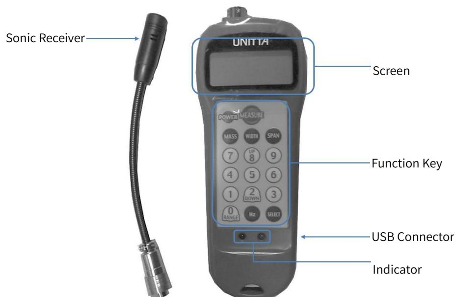
Figure 4-12 Appearance of the instrument
