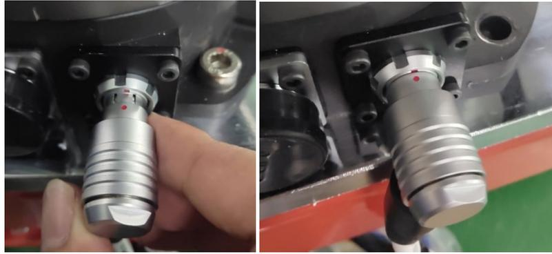
Figure 5-8 Communication cable plugging diagram
